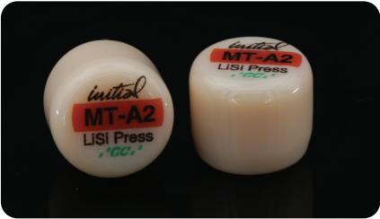
Fig. 2a: Lithium disilicate glass ceramic ingots for pressing (Initial LiSi Press ingots, GC).
