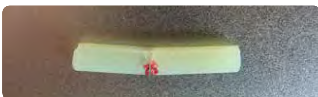
Figure 11: everX Flow sample after failure, still in one piece Source: Lyon University (LMI), France, 2019. Data on file.
