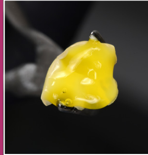
Pre-treat with 5% HF (Hydrofluoric acid) for 60 secs.
