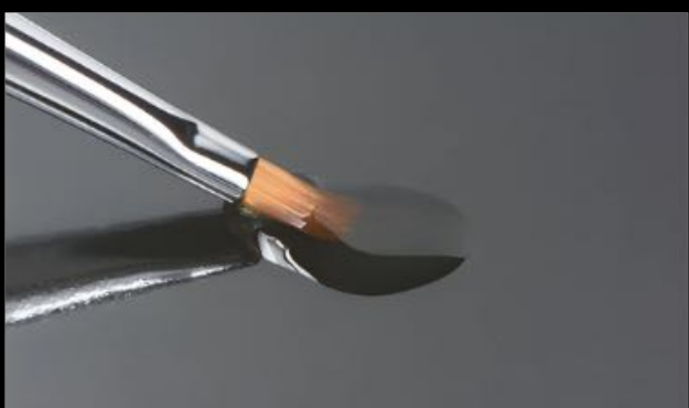
Touch the drop with the brush or instrument in order to moisten it
