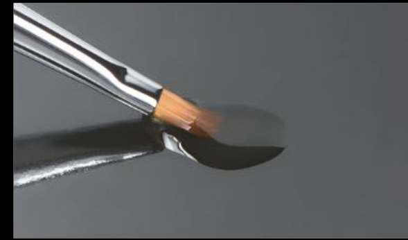
Touch the drop with the brush or instrument in order to moisten it
