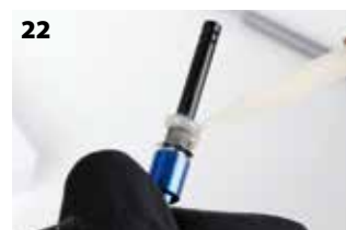
Fig. 22: The fixing material is only applied to the upper third of the gluing base.
