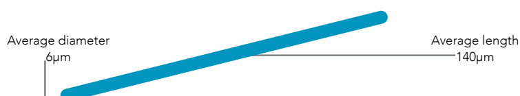
Figure 5: Optimised fibre aspect ratio
