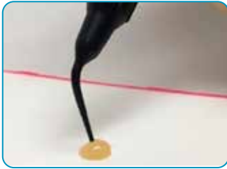
Figure 6: Flowable & thixotropic viscosity
