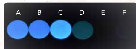
Fluorescencija - 0,5 mm pločice. A: G-CEM Veneer; B: Variolink Esthetic; C: Panavia V5; D: NX3 Nexus; E: Calibri; F: RelyX Unicem
