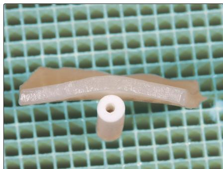
Results after 5th firing (770°C 1min, Hold). Test conducted by Masayuki Hoshi, RDT.
