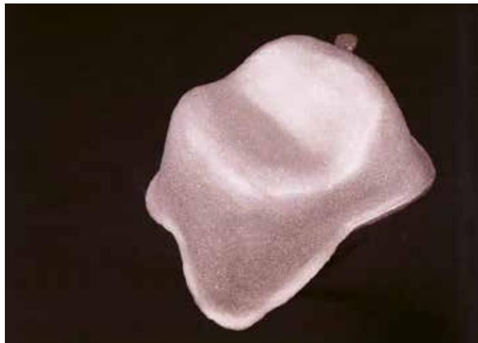
EN Remove the oxidation layer with disposable, pure 110 $\mu$  Al2O3 only and with a maximum pressure of 2 bar. Always observe the instructions for use of the corresponding alloy manufacturer. INmetalbond application, see page 30.
