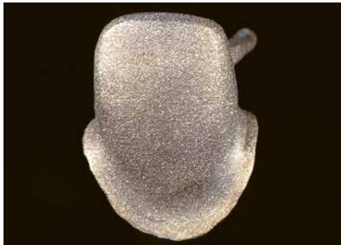
EN Cast metal frameworks are finished using tungsten carbide metal burs or ceramic-bonded grinding instruments and oxidized according to alloy manufacturer's instructions. INmetalbond application, see page 30.
