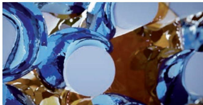
Within the IPN structure, the individually silanated E-glass fibres are surrounded by bis-GMA and PMMA.
