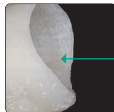
Reaction layer: Hybrid layer consisting of investment and press material
