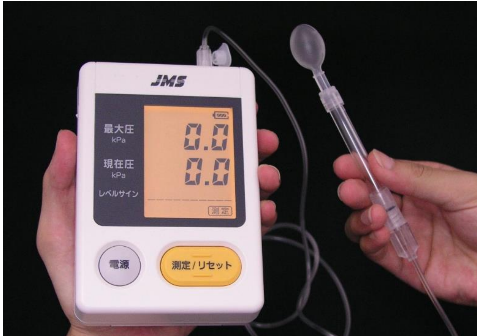
Tongue Pressure Meter (TPM-01, JMS)
